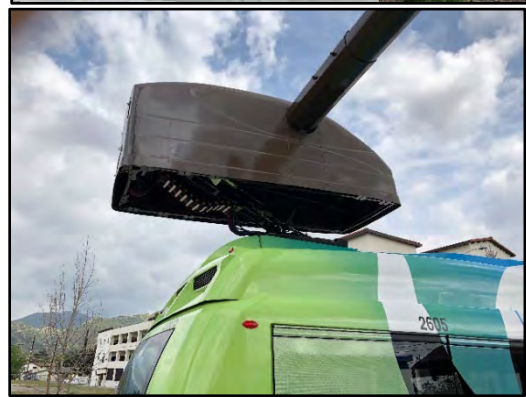
Figure 5: Overhead Pantograph Charging System
