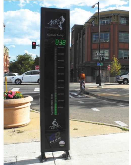
Continuous bicycle counter in Boulder, Colorado. Image Source: PeopleForBikes
