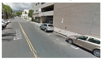
Figure 6.3: Frequent violation of the PM Tow-Away Zone was observed. However, storage space for northbound right-turn traffic appeared to be adequate despite the violations during the afternoon peak.
