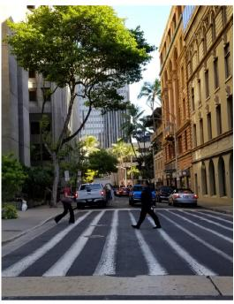
Figure 6.10: Parking violations on both sides of the street results in Merchant Street operating as a one-lane roadway.
