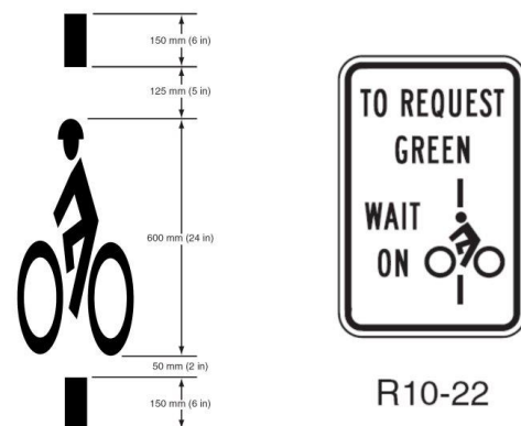
Figure 6-40: Bicycle Signal Detection Marking and Signage
