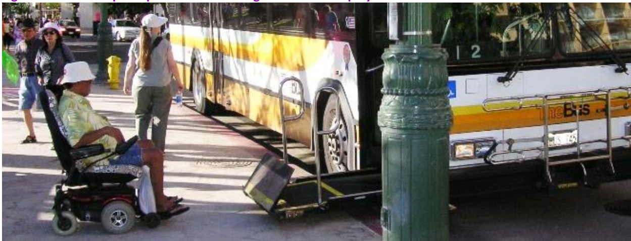
Figure 8-10: Bus Stops Require a Clear Loading Area for Lift Deployment
