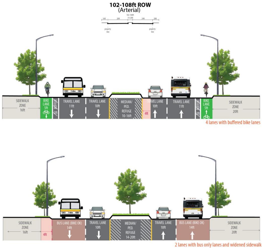
Figure 3-44: 102 to 108 Foot ROW with 14 to 20 Foot Median and 16 to 20 Foot Sidewalk
