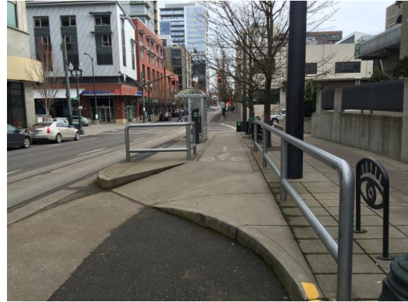
Figure 8-29: Bus Stops Should Be Integrated With Bike Lanes
