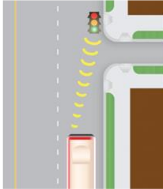
Figure 8-24: Signal-Priority Technology Can Help to Reduce Delay for Buses
