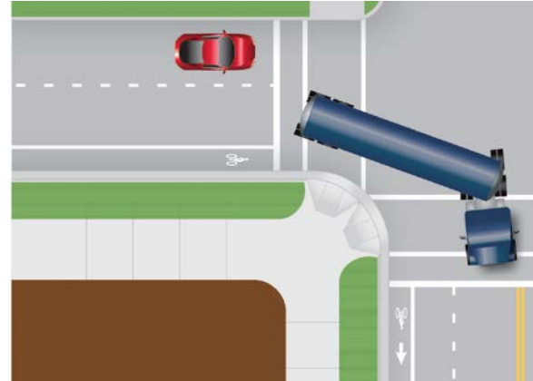
Figure 4-8: Corner Radii can be Kept Smaller by Allowing Trucks and Buses to Turn into Multiple Receiving Lanes
