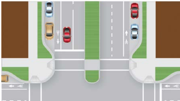
Figure 4-12: Integrating Curb Extensions and On-Street Parking into the Sidewalk Corridor Enhances Pedestrian Safety and the Walking Experience
